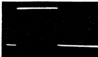
Fig. 4. Oscillogram of square wave applied to circuit under test. The vertical rise of current is too rapid to show on the plate.
